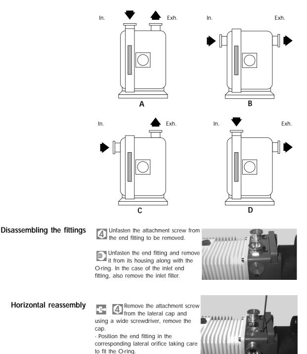
Attach the end fitting with the screw. In the case of the inlet end fitting, fit the filter at the bottom of the orifice.
