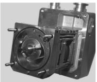
Disassembling the intermediate flange (two-stage pumps) Insert two screwdrivers in the notches and release the flange in the axis.
