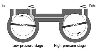
Application Two stage rotary vane pumps are the best choice for application requiring an ultimate vacuum as low as 10<sup>-3</sup> Torr (1.33 x 10<sup>-3</sup> mbar). Note : when operating a two stage vane pump continously, greater than half an hour, above 1.0 Torr, the unit should be equipped with an oil mist eliminator and oil return system, see oil draining kit (page 63), or a single stage pump should be used.
