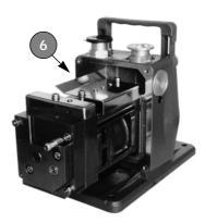
Disassembling the SD pump oil system (except 1015 SD, 1021 SD) The oil system is set in the factory, it must be reset in the event of disassembly (see reassembly). However, the rear flange (7) can be disassembled without modifying the setting. Remove the spinner-cam (8) by removing the circlip.
