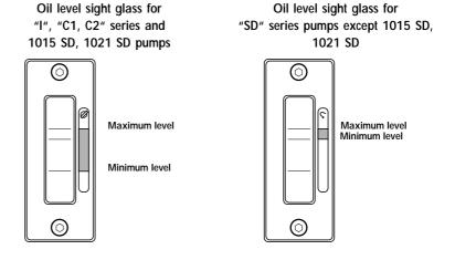
Note: Optimum pump performance and service life are obtained when the oil level is between the maximum level and the minimum level.
